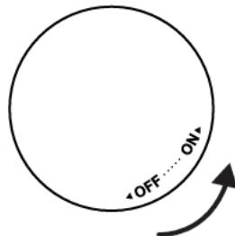
The privacy cover on the upper camera also functions as the power switch for OMNI.
