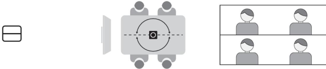
When Conversation Mode is activated, a Conversation Mode icon will appear in the top-left corner of the display and remain visible for approximately 1.5 seconds before disappearing.
