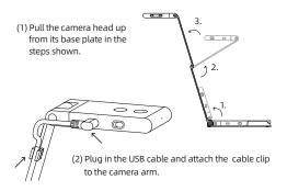
(3) Adjust the camera head until it is horizontal. Fully extend the arm to capture A3-sized content. After adjusting the camera to the desired position, press the focus button to trigger focus if auto-focus mode is off.
