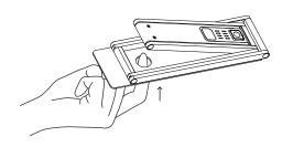
(2) Lift the other side of the arm, then pull and flip the camera head in the sequence and direction indicated by arrows below.
